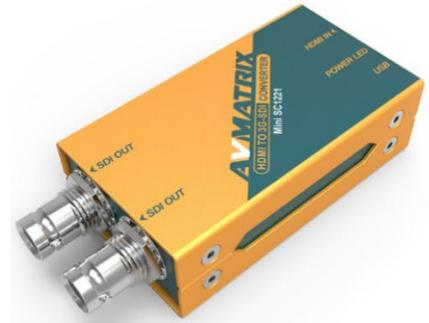
Mini SC1221 is an exquisite and portable HDMI to SDI converter. With micro USB power supply, convenient and detachable mounting bracket, MiniSC1221 is the best choice for indoors and outdoors. It adopts a type A HDMI input and dual 3G-SDI outputs, supporting a conversion of full HD resolution signal of 1080p60 to professional SDI signal. Different video rate of SD/HD/3G-SDI is selectable for SDI output.
