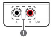
1 L/R OUT: Connect to the amplifier such as active speakers or TV with stereo RCA cables to output the received audio signal.
