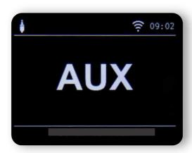
You can now play music from the external device. The output (skip track, back, stop, play) is controlled via the connected device. The volume can be adjusted via the **VOL+** / **VOL-** buttons or the control knob on the radio or via the external device. Please note that you have to connect the external device using a suitable cable.
