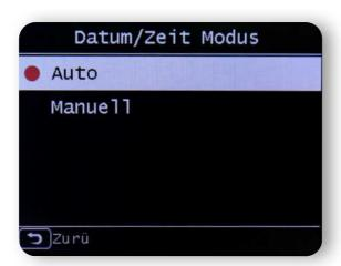
The device's factory setting is to automatically set the time. If the device is connected to the internet via the network, the time and date are automatically synchronised. You therefore do not have to set the time manually. You can change these settings at any time in the main menu under System.
