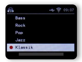
Use the ▼ ▲ buttons on the remote control or the control knob on the device to select a sound preset and confirm by pressing **OK** on the remote control or by pressing the knob on the device.
