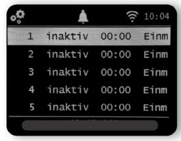
Select one of the 5 available alarms and confirm by pressing the **knob** on the device or the **OK button** on the remote control.
