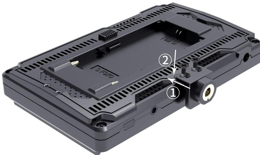
① Fasten the 1/4" screw lock with the monitor.
