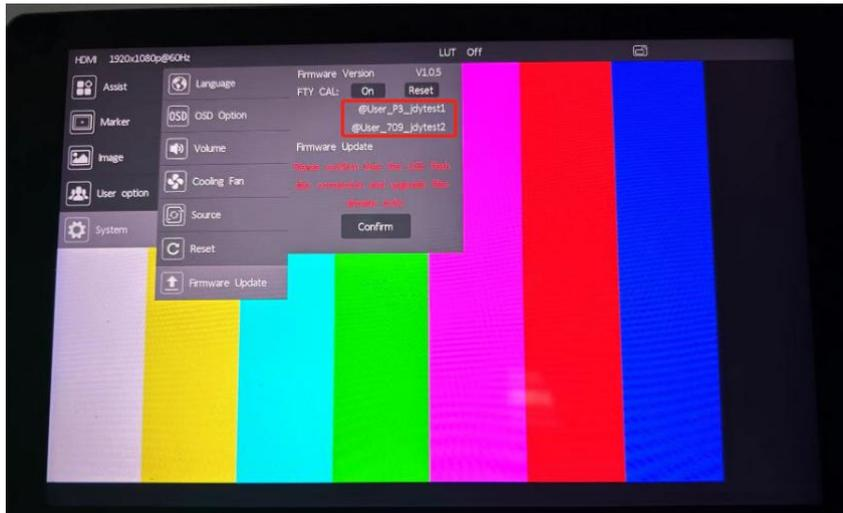
5.4 If you import your own LUT calibration but encounter abnormalities or poor result, you can clear the calibration LUT by clicking "Reset" in FTY CAL and return to the factory calibration.
