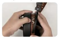
1. Locate the connection point between the earpad and the headphone body;
