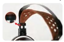
1. Locate the adjustment screw hole on the side of the slider and use a hex screwdriver to adjust the dampling force;
