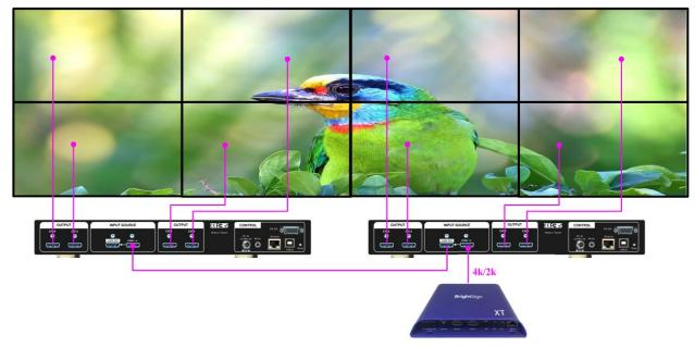
3.3 If Loop out port has not been used, user can use loop out port to connect with monitoring system in control room to see the status of the video wall content.
