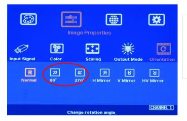
Use [Orientation] menu to rotate images in TV2 and TV3 to display the same image direction.
