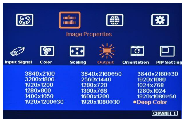
Select output resolution and 10-bit deep color output
