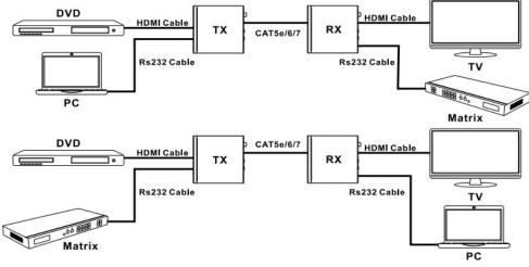
6.4 Bidirectional Ethernet signal Application Example
