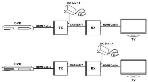
6.2 Bidirectional Infrared control Application Example
