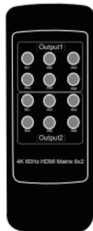
1) The 6 buttons on Output 1 is the corresponding input source IN1-IN6 which out from Output 1, IN1-IN6 can be switched freely.
