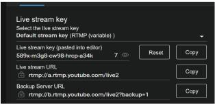
Click the cicen to obtain the URL of the RTMPS push stream, according to the following information, the RTMPS push stream URL is rtmps://a.rtmps.youtube.com/live2/589x-m3g8-cw98-hrcp-a34k
