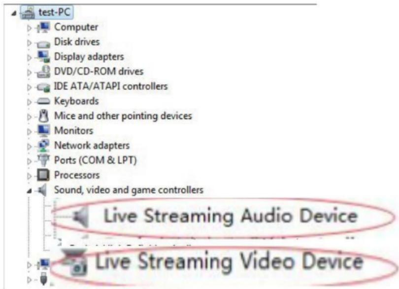
Please make sure Live Streaming Audio Device and Live Video Device has been installed.
