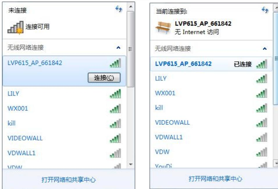
Configuring network be automatically obtain IP address and DNS server address, show as the picture below:
