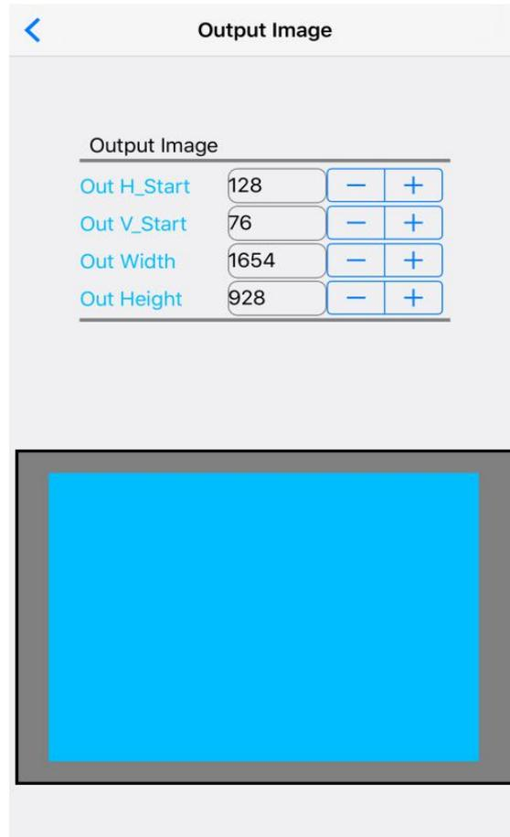
The interface is used to set the location and size of output image, user could enter parameter manually, then through **+** and **-** to adjust parameters, in diagram area of output parameters, through multiple-point touching to zoom in or zoom out image size, single-point touching to drag and adjust image location.
