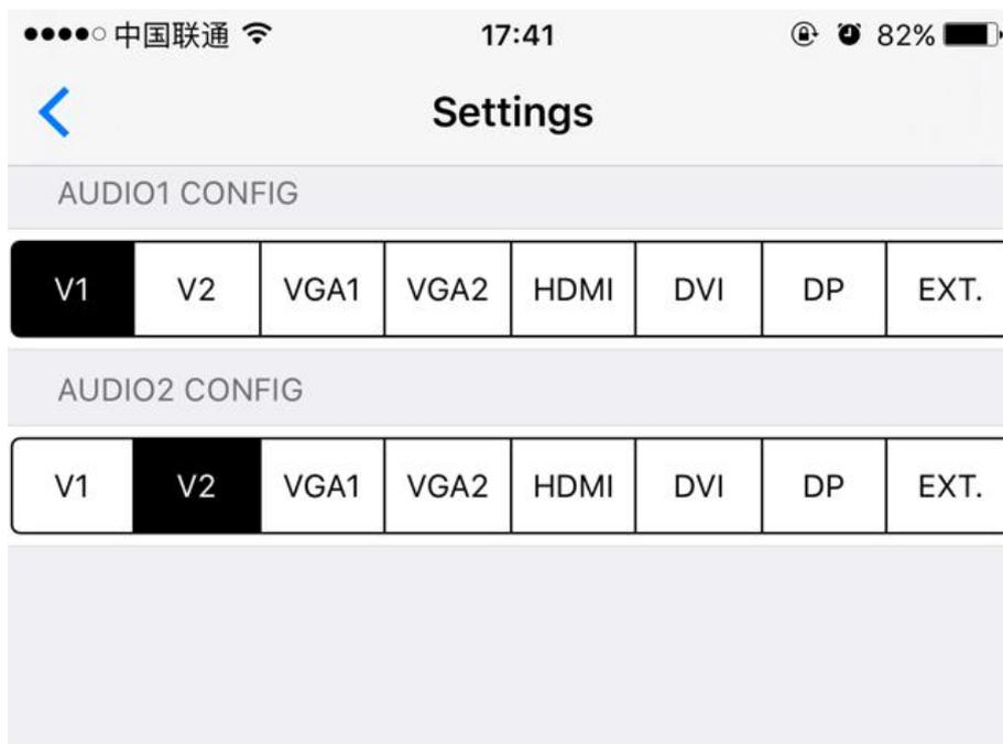
Audio setting interface could set LVP615's corresponding input signals of two audio inputs, in order to achieve audio and video synchronous switch.
