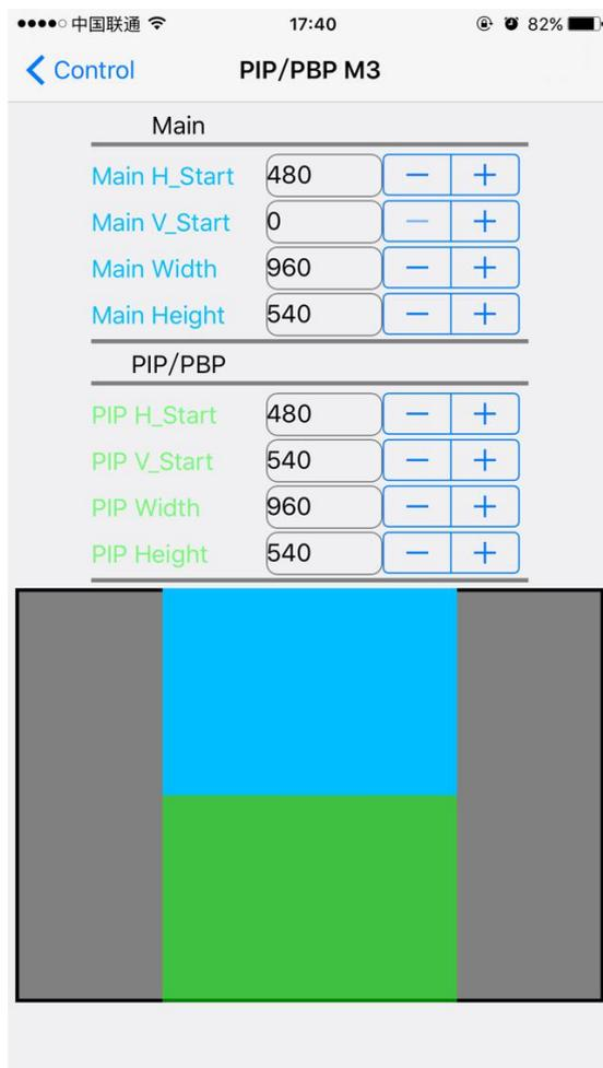
User can input specific parameters of main window and PIP window. Press and to adjust.
