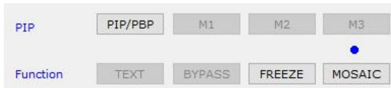
**TEXT**:text overlay display switch, used open or close text overlay function; meanwhile the bright point above the button indicates the function is open or not.
