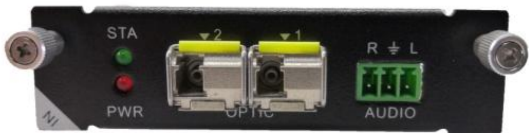
1 Port OPTIC input card with analog audio embedding.
