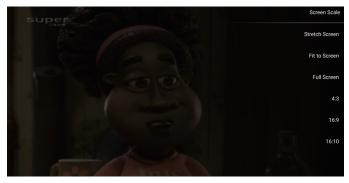
20. Select Screen Scale can switch to different display ratio.
