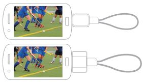
Connect PadTV to your device mirco usb or Type-c port Note:Your Android device must has USB-OTG function 1. Once PadTV HD is open, you will first need to scan for TV channels, click on menu
