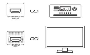
Note: The dual-port output mode is suitable for AV receivers that do not support resolutions higher than 4K or 3D functionality, and when the display device supports resolutions higher than 4K or 3D functionality.
