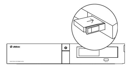
Note: Do not load or replace the hard disk while the device is powered on to avoid damage to the device or hard disk data. Brand new hard disks need to be formatted before loading. This device supports the following hard drive formats: EXT3, EXT4, NTFS, FAT32, EXFAT.
