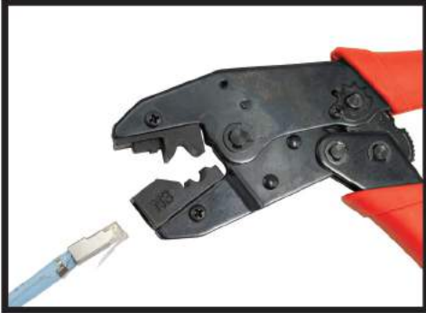
Put the 106A Plug into the crimp tool in the right position
