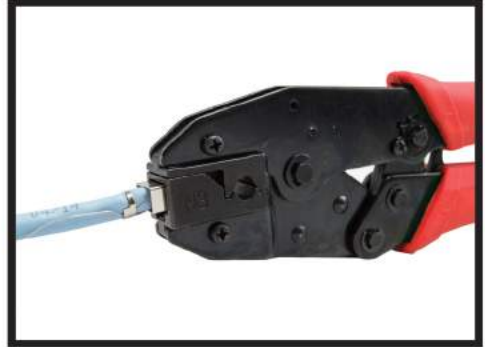
Squeeze the tool to push the contact blades into correct positions
