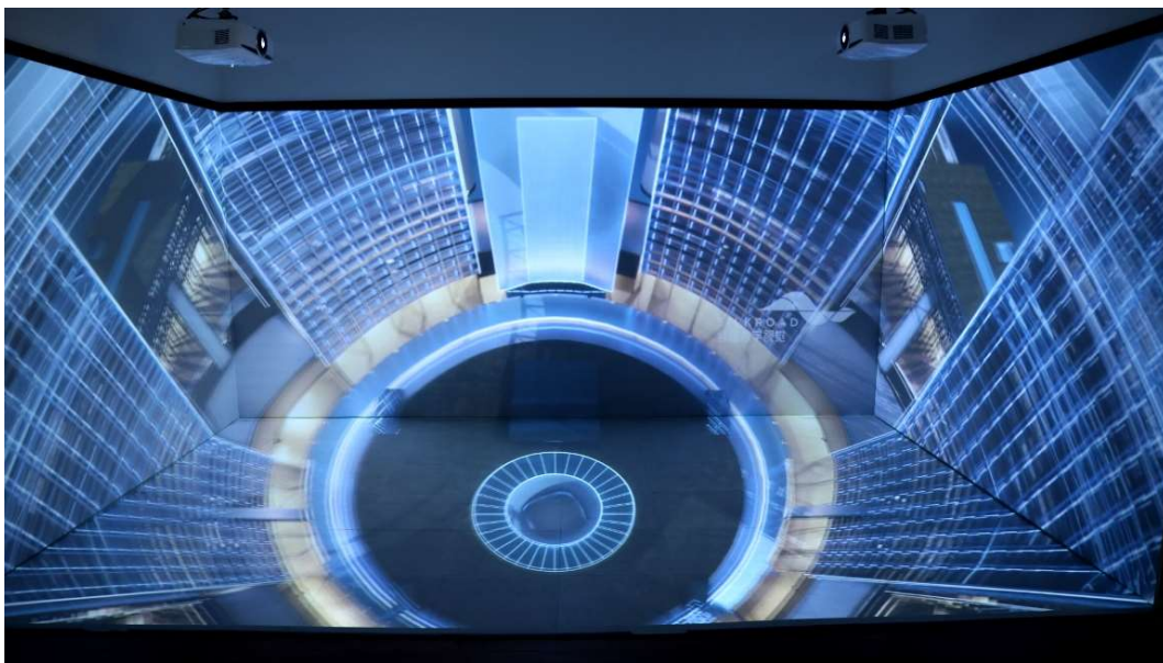
Immersive system with 3 walls and one floor
