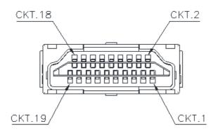
**HDMI Type A Connector Pin Assignment**
