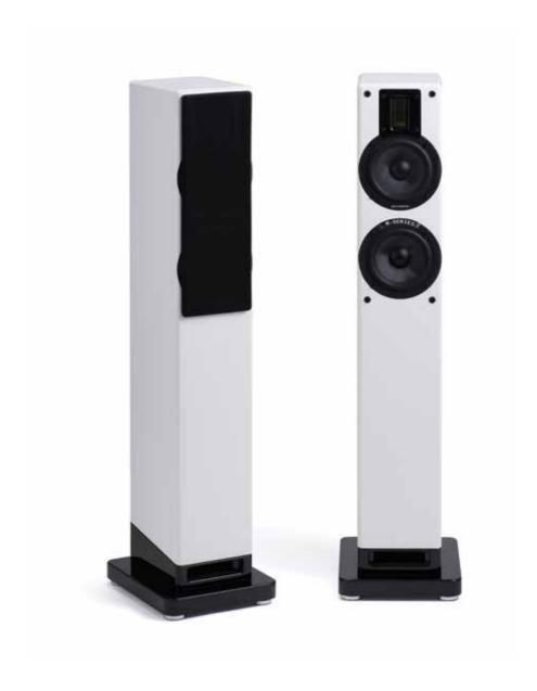
The M-6 is a compact, 2.5-way, floorstanding speaker. The speaker is designed around an ultralight ribbon planar tweeter and two paper-polypropylene compound bass-midrange drivers. The bass driver assists up to app. 300 Hz for added bass capability.
