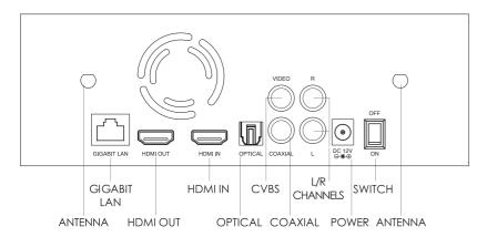
Instruction to installation of the antenna: Please insert the two antennas in the parcel into the antenna ports in the above diagram.
