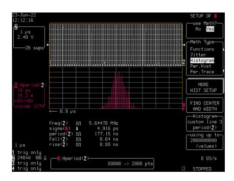
FifoPiMa SCK (5.6448MHz) jitter is measured 4.49ps RMS (noise floor excluded)
