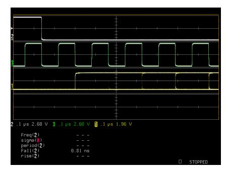
Under a 1GHz bandwidth 8Gs sampling digital oscilloscope, the quality of the FifoPiMs output signals is almost perfect. The noise levels are very low. No overshoot and no ring. There is also no ripple over the logic levels. The eye diagram of the DATA signal looks great. Both LRCK and DATA signals are precisely aligned to the falling edges of the SCK. FifoPiMa's output signal quality could be so far the best.
