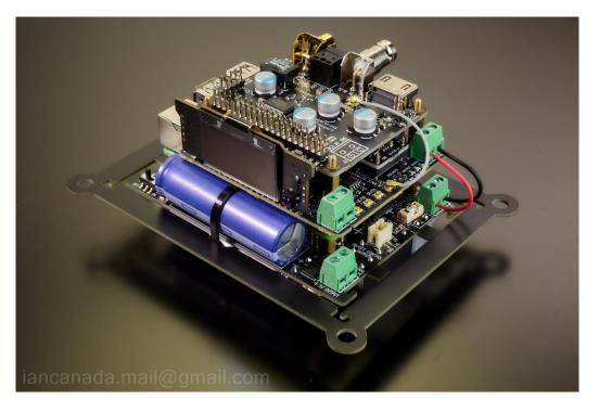
5. Install two 18650 3.2V LifePO4 battery cells into the battery holders at the bottom side of the PurePi. Please be very careful not to reverse the battery cells.
