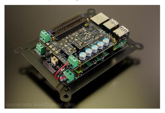
4. Install a TransportPi MkII (or HdmiPi, HdmiPi Pro, TransportPi AES) on top of the FifoPiMa using 4 13mm standoffs. Connect the supplied U.FL cable from FifoPiMa MCLK output socket to J4 MCLKIN of TransportPi. Install a MonitorPi into the AUX GPIO of FifoPiMa if you need a OLED display (optional).
