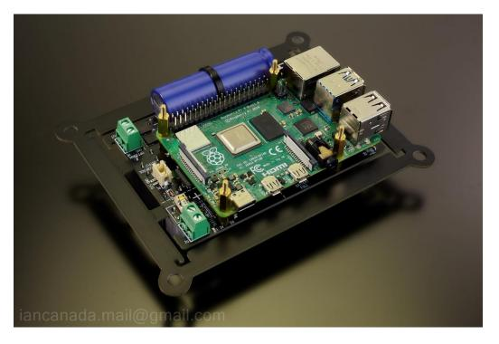
3. Install a FifoPiMa (or a FifoPiQ7, or other audio HATs) on top of the Raspberry Pi properly. Use two good quality wires connect the pure 3.3V battery power output from J2 of PurePi to J5 of FifoPiMa. Please be very careful not to reverse the positive and negative terminals.
