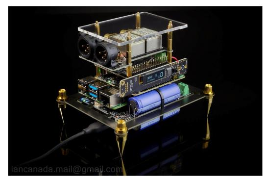
3. ESS DAC in SYNC clock mode with balanced/SE transformer I/V
