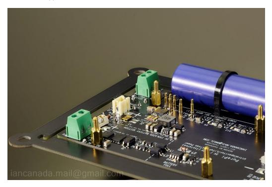
Install Raspberry Pi on top of the PurePi through the 7mm standoffs and then 4 11mm standoffs to fix it at the position. Make sure the five spring contacts are connected to the GPIO pins properly at the bottom side of the Raspberry Pi.
